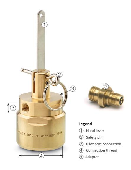
The manual/pneumatic release device allows manual or pneumatic actuation of multiple highpressure cylinders in series, which are connected to the master high pressure cylinder by a pilot hose.
